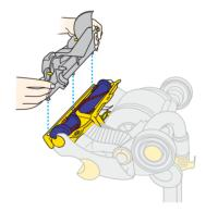
Rest the three tabs on inside of bumper strip and secure soleplate back into position.
