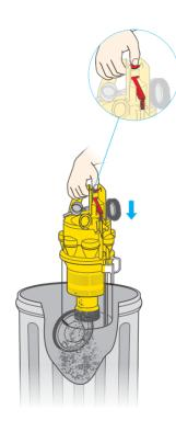
Push the red bin emptying button as shown to release the bin base and empty directly into trash.
