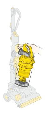
Empty the Clear bin™ as soon as the MAX mark is reached. Press cyclone release button to release cyclone from machine.
