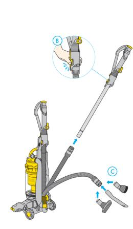
**B** To fit tools directly to hose, first extend the wand. Then press side buttons to remove wand handle from the hose.
