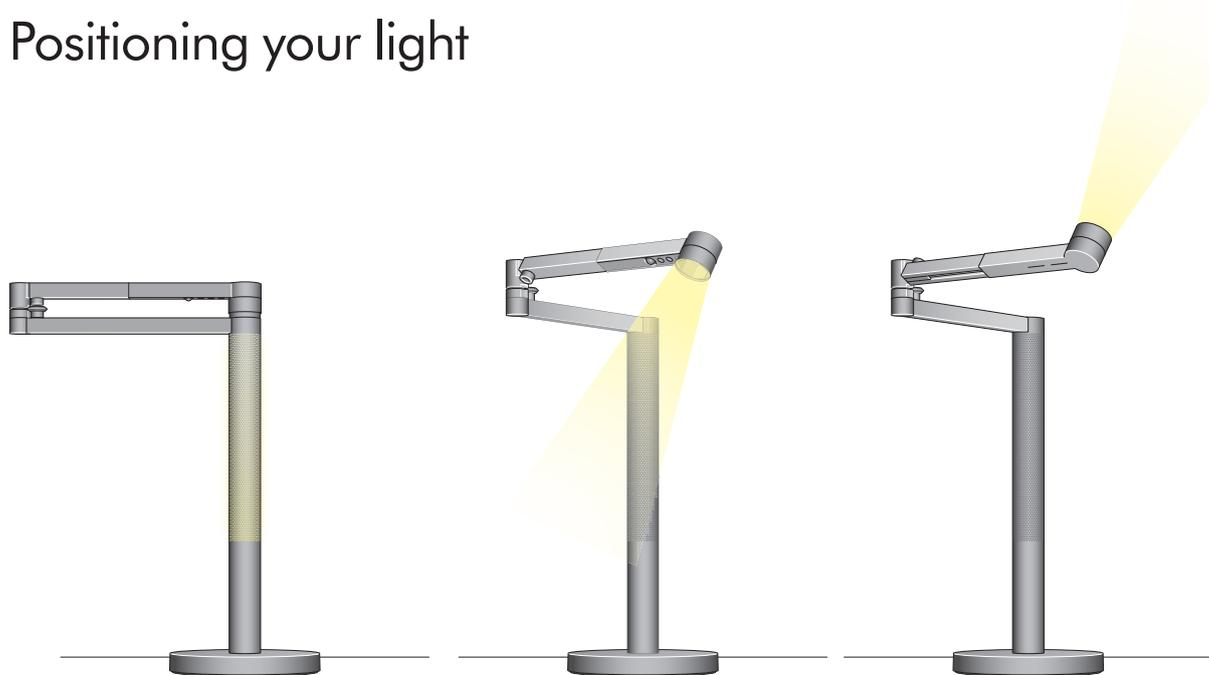
You can easily change the position of your light by independently rotating the optical head, arm and stem up to 360°.
